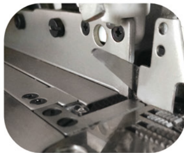
斩刀结构 Cutter structure
