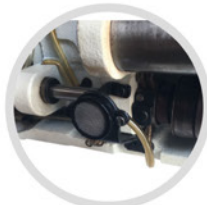
柱塞泵润滑 Plunger pump lubrication
