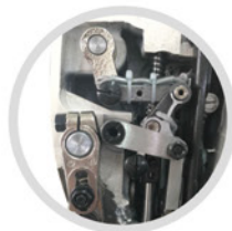
新连杆机构 (杜绝提升压脚上下不灵活现象) New connecting rod mechanism (Put an end to the flexible operatillity of foot lift up and down )
