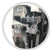
新连杆机构 (杜绝提升压脚上下不灵活现象) New connecting rod mechanism (Put an end to the flexible operability of foot lift up and down)
